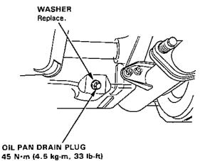
Reinstall the drain plug with a new washer, and refill with the recommended oil.
