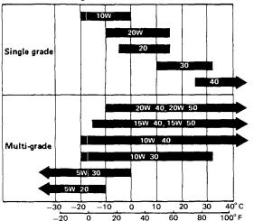
Engine oil viscosity for ambient temperature ranges.
