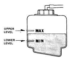
Supply the coolant reservoir tank with coolant to "MAX", if the coolant level is lower than "MIN" or near to "MIX".
