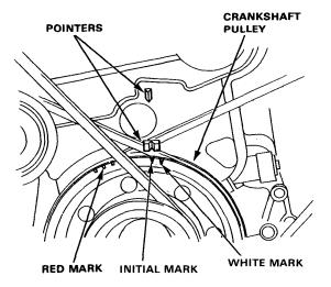
11. Read initial timing when initial timing mark is aligned to the pointer.
