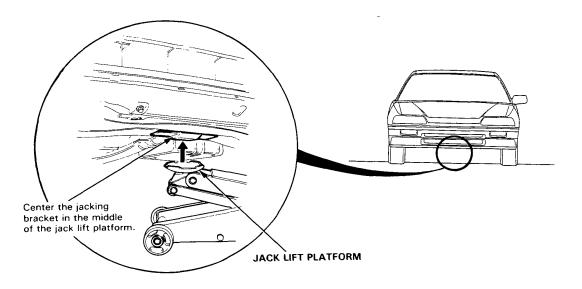
Center the jacking bracket in the middle of the jack lift platform.
