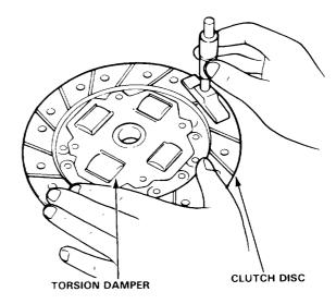
Measure the clutch plate runout with the mainshaft and a dial indicator.
