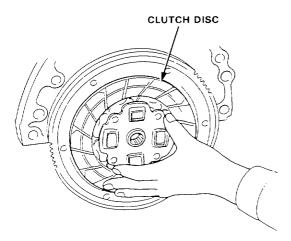
2. Measure the clutch disc thickness.
