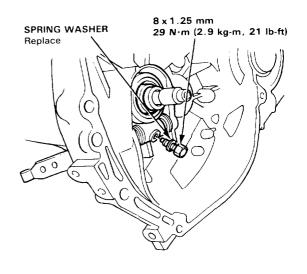
Move the release arm up and down to make sure the fork fits properly against the bearing, and that the bearing slides freely.
