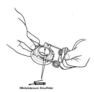
2. Install the release arm clip in the locating holes as shown.
