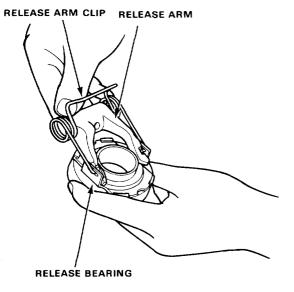
Install the release shaft and the release bearing.
