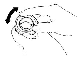
Replace the bearing with a new one if there is excessive play.
