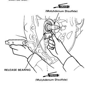
4. Align the release shaft and release arm, then install a new spring washer and bolt.
