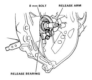
Separate the release arm from the bearing by removing the clip from the holes in the release bearing.
