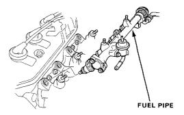
Align the center line on the connector with the mark on the fuel pipe.
