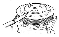
NOTE: The shims are available in two sizes: 0.2 mm and 0.5 mm of thickness.
