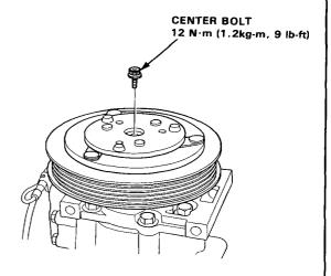
Remove the pressure plate and shim(s) taking care not to lose the shims.
