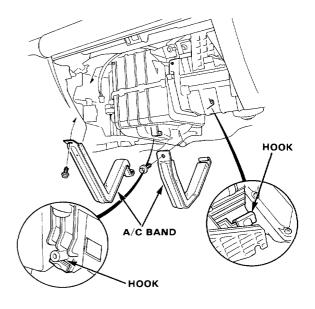
7. Remove the mounting bolts (2) and evaporator.
