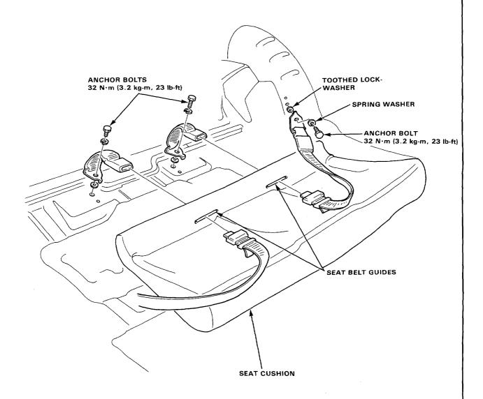
4. Install the seat belt in the reverse order of removal.
