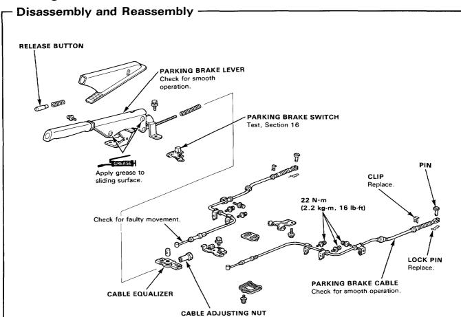
Disconnect the parking brake cable from the lever on the rear caliper by removing the lock pin and pin.
