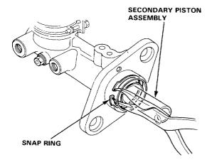
Remove the stop bolt while pushing in the secondary piston assembly.
