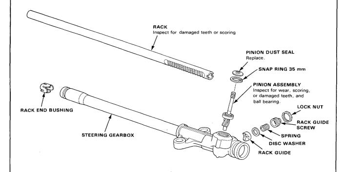
NOTE: The pinion assembly bearing cannot be removed. If the bearing must be replaced, replace as an assembly.
