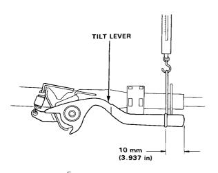
10. If the force measured is not within the specification, remove the tilt lock plate then reset it in the position where the correct force can be obtained.
