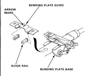
Loosely install the steering column assembly with the nuts, bolts and lower column bracket.
