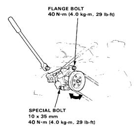
Start the engine and turn the steering wheel from lock-to-lock several times, then recheck the belt tension.
