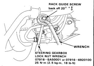
Tighten the guide screw until it compresses the spring and seats against the guide, then loosen it.
