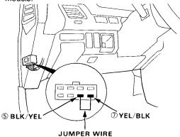
Check that battery voltage is available at the fuel pump connector when the ignition switch is turned ON (positive probe to the YEL/BLK wire, negative probe to the BLK wire).
