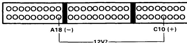
Measure voltage between C10 (+) terminal and A18 (-) terminal.
