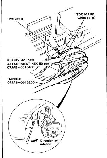
NOTE: If the pully bolt loosens while turning the crank, retorque it to 120 N·m(12.0 kg-m, 87 lb-ft).
