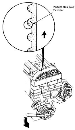
Rotate pulley and inspect belt
