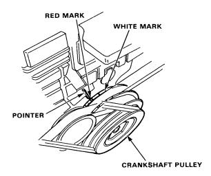
Adjust as necessary by loosening the distributor adjusting bolts, and turn the distributor housing counter clockwise to advance the timing, or clockwise to retard the timing.
