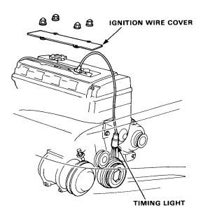
4. Adjust ignition timing, if necessary, to the following specifications:
