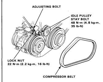
Remove the compressor mounting bolts (4) and compressor. Rest the compressor on the front beam.
