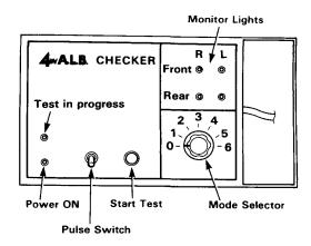
With the transmission in neutral, rotate each wheel briskly (one revolution per second) by hand and confirm that its respective monitor light on the checker blinks as the wheel rotares.
