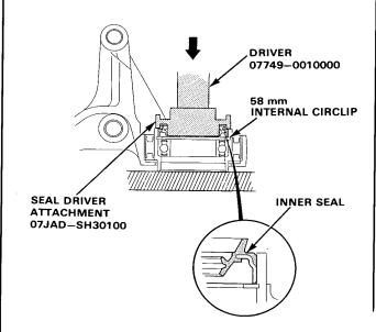
4. Press the intermediate shaft into the shaft bearing.
