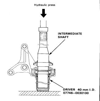
Seat the 38 mm external circlip in the groove of the intermediate shaft.
